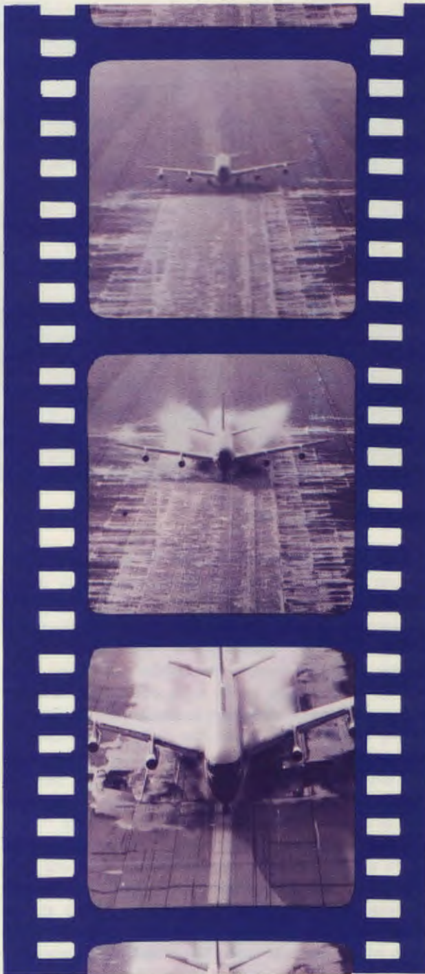
Sequence taken during NASA hydroplaning tests.
